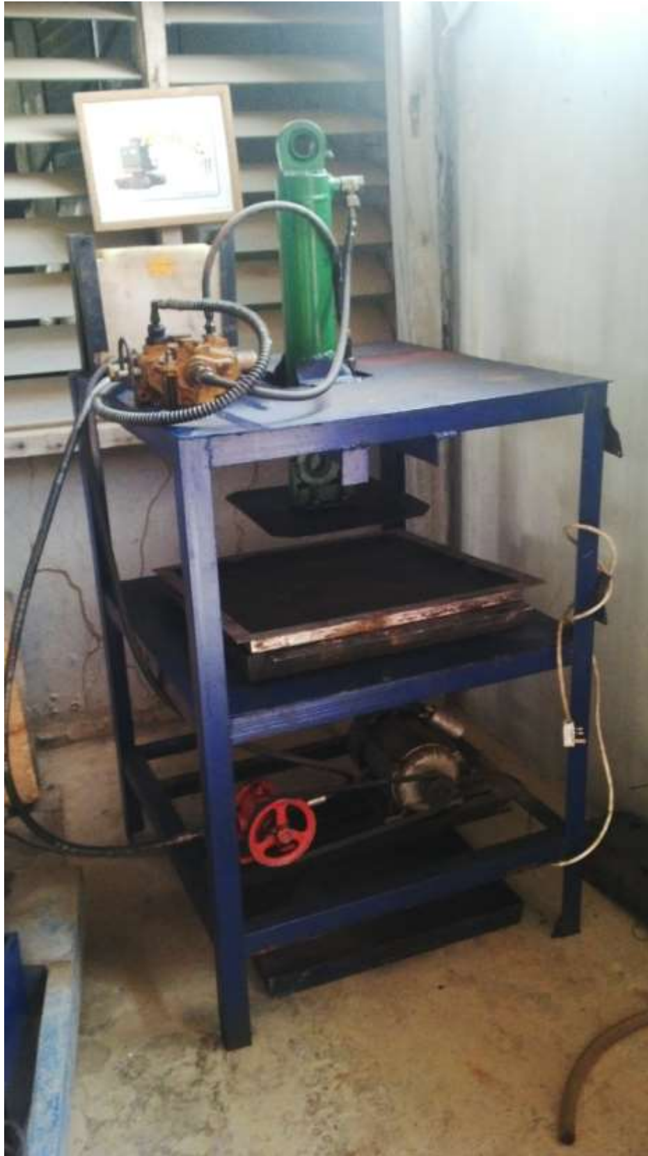
Figure 8. The ceiling board making machine
