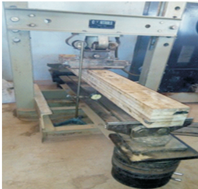
Figure 1: Two point static bending test setup
