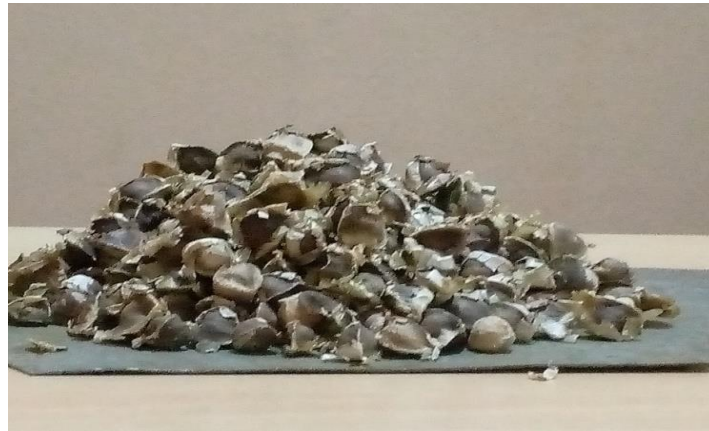
Figure 3. Determination of angle of repose on galvanized steel
