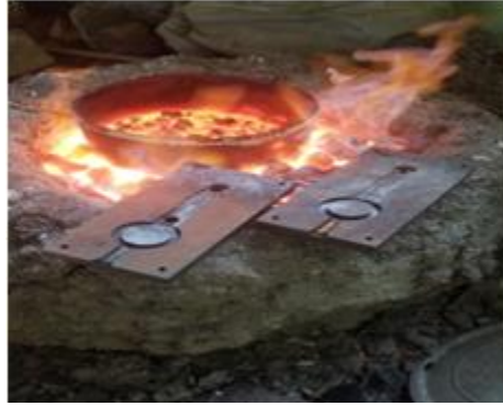
Plate 5. Preheating of the mould
