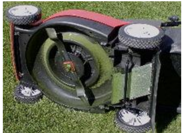
Figure 2. A rotary mower (viewed from underneath), with a mulching blade that rotates
