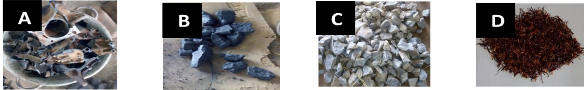
Plate 1(A-D). Auto parts scrap, ferrosilicon (FeSi), limestone, and copper respectively used for grey cast iron sample production
