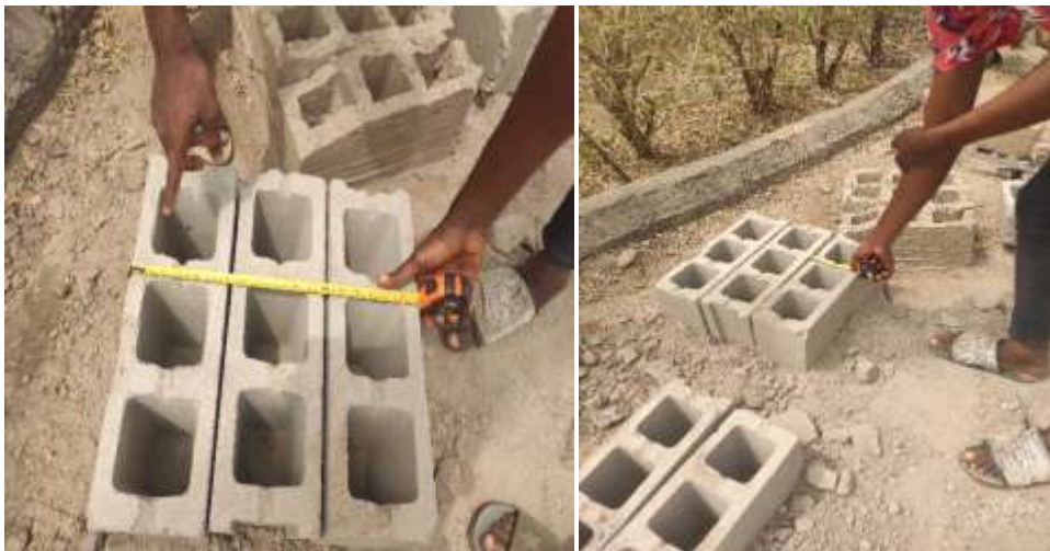
Plate 2. Arrangement of the blocks in the platform
