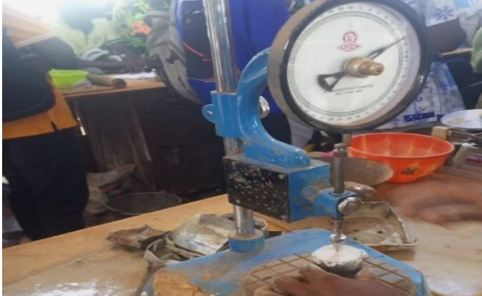
Plate 4: Liquid limit, Using Cone-Penetrometer
