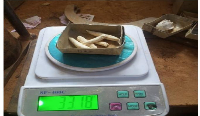
Plate 6: Determination of plastic limit of the Kaolin Clay
