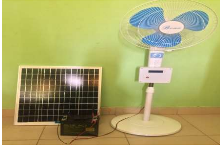
Figure 5: Complete Solar DC Fan with Controller (Smart Ventilator)
